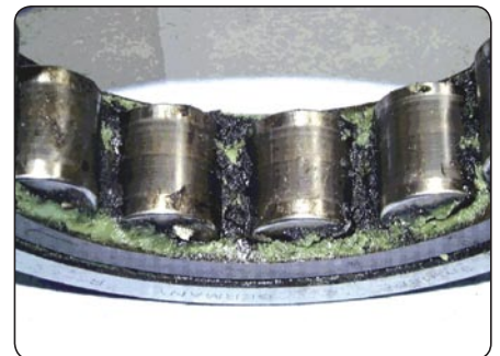
Lubricant degradation caused by electrical discharge currents
